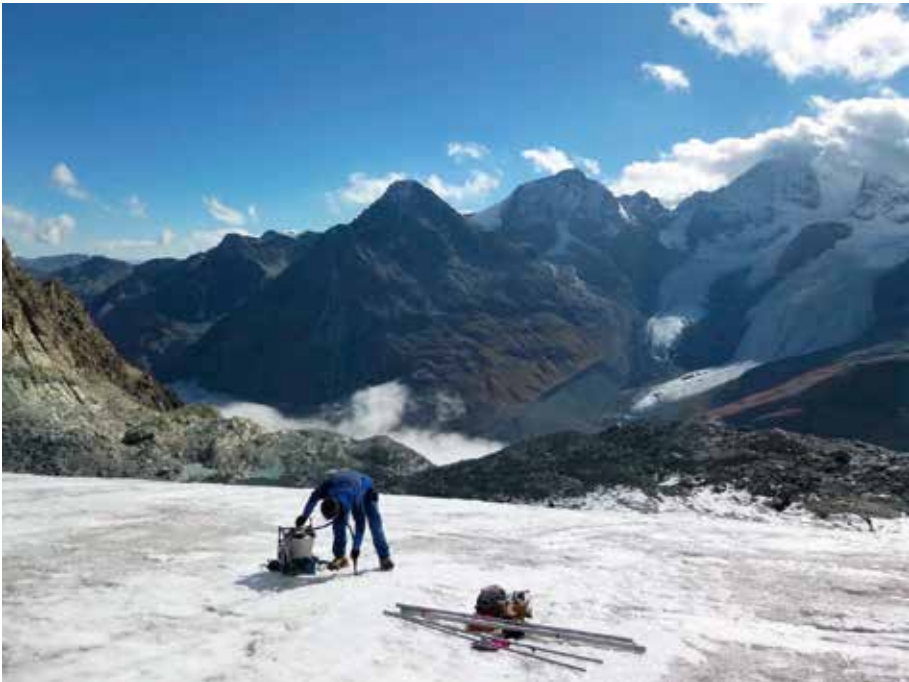
Installation of an ablation stake using a steam drill on Vadret dal Murtèl in September 2015 with Vadret dal Tschierva visible in the background. (Photo: M. Huss)
