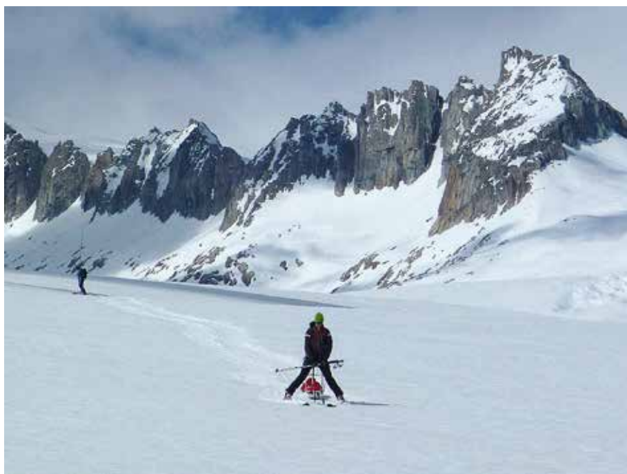
Snow depth survey using traditional hand-probes (background) and ground penetrating radar (foreground) (Photo: M. Huss)
