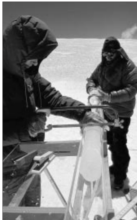
Photo 6.6: The sawing up and packing of the ice cores on the Cerro Tapado in the Chilean Andes. (Photo: P. Gino)
