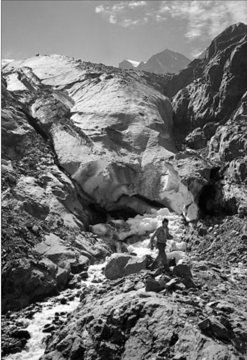
Photo 4.1: In order to obtain measurements of the terminus of the Glacier de Corbassière (VS) which cannot be measured directly, a fixed point is marked on the protruding rock and the terminus measured from this point. Photogrammetric surveys of the glacier terminus have been conducted since 1998. (Photo: D. Vonder Mühll)
