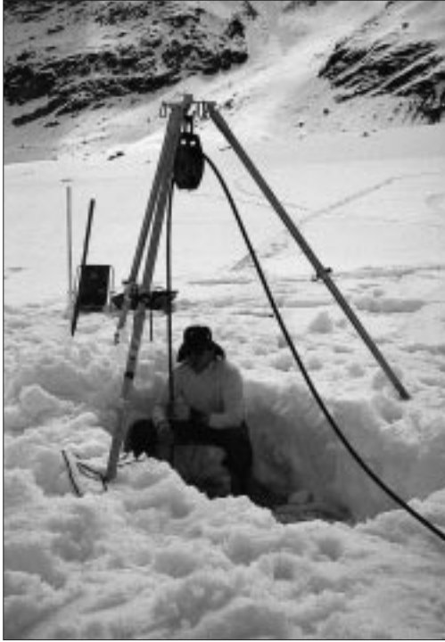
Photo 6.5: Hot-water drilling on the Unteraargletscher. (Photo: M. Lüthi)
