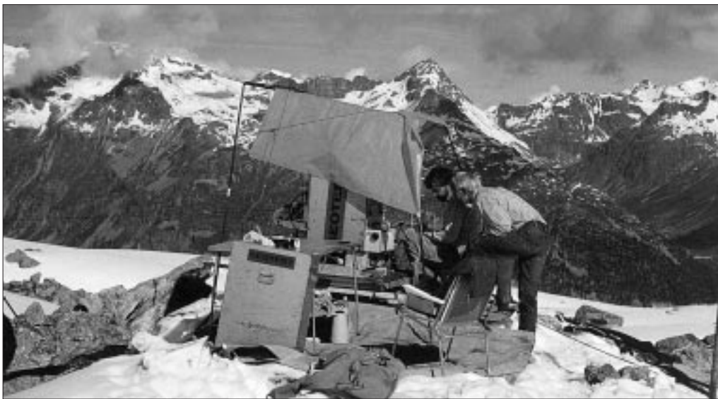
Photo 6.3: Borehole geophysics at the Murtèl-Corvatsch site: The physical variables alongside the boreholes are recorded (e.g. \gamma\text{-}\gamma - log). (Photo: D. Vonder Mühll)
